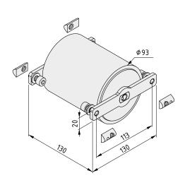
Strong braking action for lifts Robust steel axle Carries weights up to 25 kg
