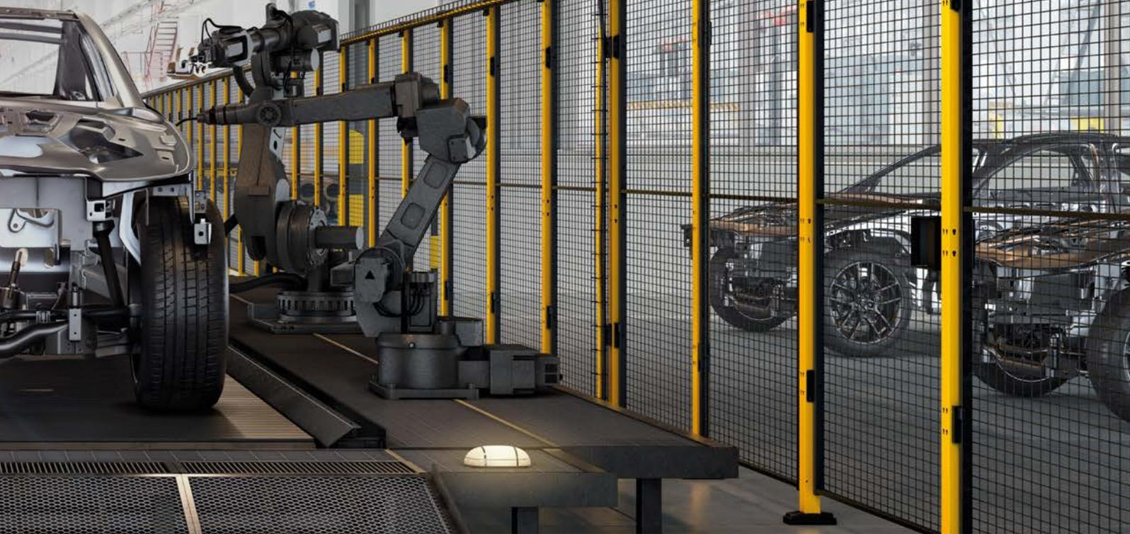
Steel protective fencing and safety elements from the Swedish manufacturer Axelent AB are designed to secure production lines, robotic workplaces, warehouse areas and places where injuries to operators must be prevented. If required, version in aluminium profiles can also be offered.
