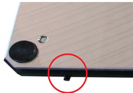
Workpiece carrier with shock absorber
