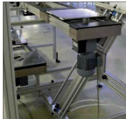
Inclined transfersystem lift-upper or basement type
