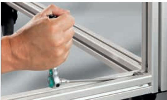
Key Inserts from item feature long wrenches and special head shapes. They enable optimum power transmission whether they're used vertically or at an angle. The Key Inserts can be used with the relevant item Ratchet Wrenches. Variants with a 1/4" square drive fit standard torque wrenches.
