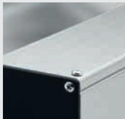
Wall Profiles and Lid Profiles can be secured in position by means of Self-Tapping Screw St 4.2x9.5. The Support Profiles must be provided with a bore  $\varnothing$  3.5 mm in the marking groove for this purpose. The screw connection creates a conductive bond between the conduit elements.
