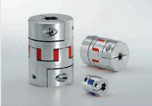
Couplings can be installed between the mechanical drive elements (Timing-Belt Reverse Units, chain drives, Ball Screw Units, Bevel Gearboxes) and the drive in order to suppress and compensate for angular errors and radial or axial offset.
