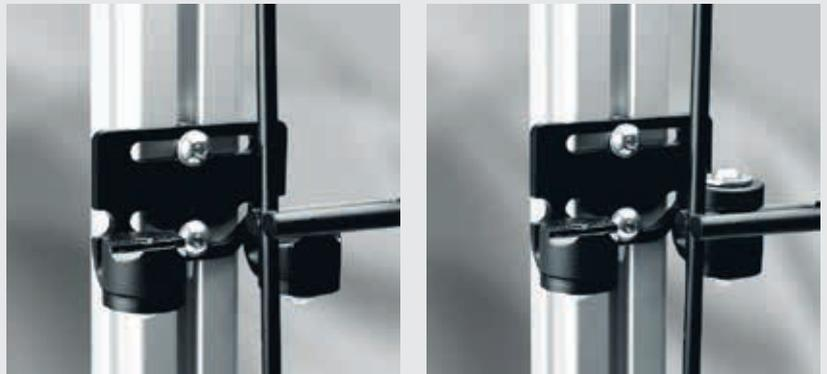
The Dual-Rod Mesh is first hung from a preassembled Dual-Rod Mesh Hanger, and then screwed into position with further Hangers. Recommended spacing of Hangers: 3 section heights, corresponding to 600 mm.
