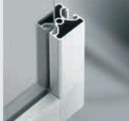
The Clamp-Profile Fastener can be combined with any desired Profiles 6 30x30 or 8 40x40 and also with the existing Clamp Profiles 6 30x30 or 8 40x40. The fact that the Clamp-Profile Fastener has a special cavity means that the panels to be fitted in the profile grooves do not need to be notched.
