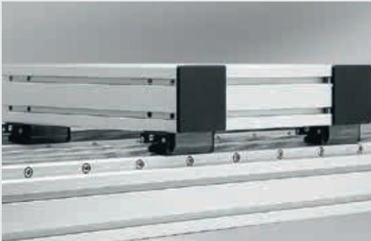
Guide systems with parallel rails on a single supporting profile can be constructed on the profile groove without elaborate alignment measures due to the special fastening geometry employed by the rail. The use of parallel rails on independent profiles or different support constructions will require the amount of alignment and fastening which is typical for profile rail guides (machining of location surfaces, use of parallel segments etc.).
