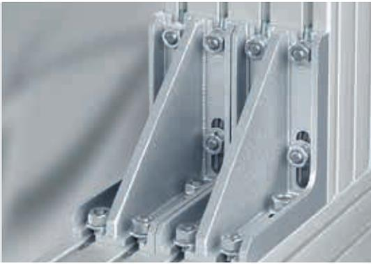
Angle Bracket 8 160x160 St M12 is used for screw attachment with Fasteners 8 M12. A particularly heavy-duty connection is possible for the profiles by using an M12 bolt with Profile 8 grooves. Alternatively, Angle Bracket 8 St M12 can also be screw attached using bolts and T-Slot Nuts 8 St M8.
