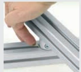
**Dismantling:** Loosen the tensioning screw, lift the locking strip out of the profile groove and swivel it back. The CLICK-Fastening Set does not need to be taken apart and is immediately ready for use again.
