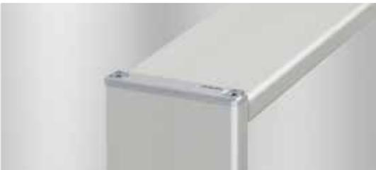
Cap 8 80x16 Zn is fixed to Profiles 8 80x16 using the enclosed screws to create a secure and friction-based connection, which ensures it can resist impacts and vibration over long-term use. A thread must be tapped into both screw channels of the flat profiles.
