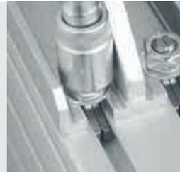
Two-part Fastener for heavy-duty securing of parts to the Profile 8 groove. The two halves of the Fastener are fitted into the groove at any point where they are then slid together. The integrated spring ball holds the Fastener in place and facilitates screw attachment.
