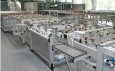
The MB Building Kit System from item is a tried-and-tested basis for machines and systems of all sizes. Profiles 8 are the most frequently used profiles of all the lines world-wide. Thanks to their design, these aluminium profiles are light, robust and versatile with a service life of many years. Due to the wide selection of modules available, Profiles 8 can satisfy virtually all your construction needs.
