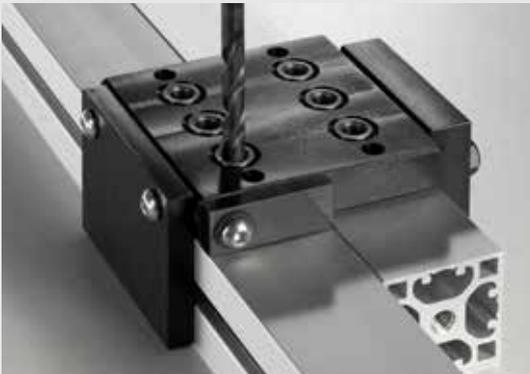
Because Drilling Jig 8 80, Standard Fastener 8 clamps to the outside of a profile, it can also be used on profiles with closed grooves. Suitable for Profiles 8 and Profiles X 8 up to a width of 80 mm.
