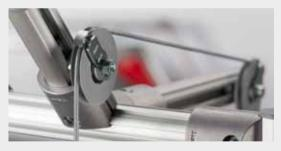
Cables often need to be redirected to create compact and efficient constructions. The Cable Pulley Wheel D42/D6-12 offers simple and secure guidance for cables. This high-quality, ball-bearing pulley can be screwed directly to the profile with or without Spacer Bushings. The bracket plate included in the scope of supply stops the cable from springing out of the pulley.
