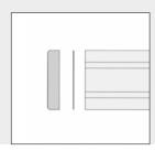
Self-adhesive Seal 8 80x40 PE (0.0.420.80) must be fitted between the profile and Pneumatic Connecting Plate 8 80x40 G3/8.
