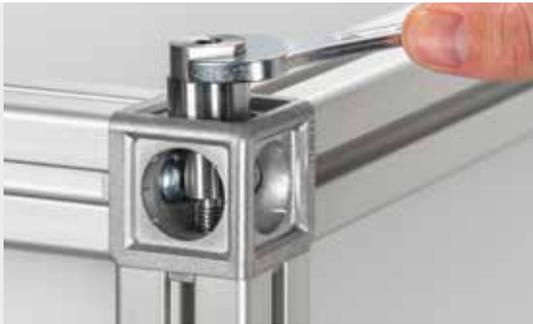
Threaded Insert M8 for Cube Fastening Set 8 is screwed into cube fastener 2D or 3D using a spanner. Its strong M8 thread can be used to fasten castors, Adjustable Feet or accessories in place. Install the Threaded Insert in the relevant profile instead of one of the Button-Head Screws supplied with the Cube Fastening Set but using a Washer from the set.
