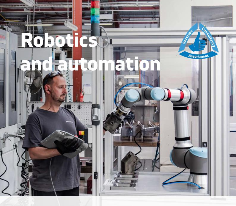
Universal Robots' collaborative robots will help streamline and automate production and relieve employees from routine work activities. Ergoswiss lifting systems contribute to ergonomic solutions where height adjustability is required. Karakuri represents simple, low-cost automation using only physical principles without an external power source.
