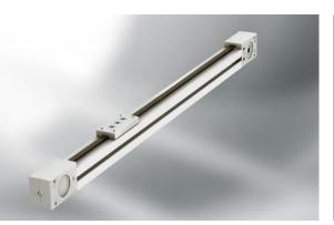
Light, quiet and high-performance! Linear Unit GSF 8 40 R10 is an efficient turnkey system with minimal space requirements. This economic Linear Unit uses only a few components to deliver maximum performance. For example, the carriage uses a Line 8 groove on the support profile as its guide. It runs without lubricants on a wear-resistant sliding shoe.
