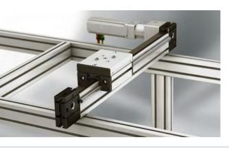
Fast speed, streamlined dimensions and high payload – all are features of Linear Units LRE 8 D10. The carriage measures just 120 mm wide and is guided securely along steel shafts by roller elements. The carriage has a flat surface for accommodating application-specific mounting holes.
