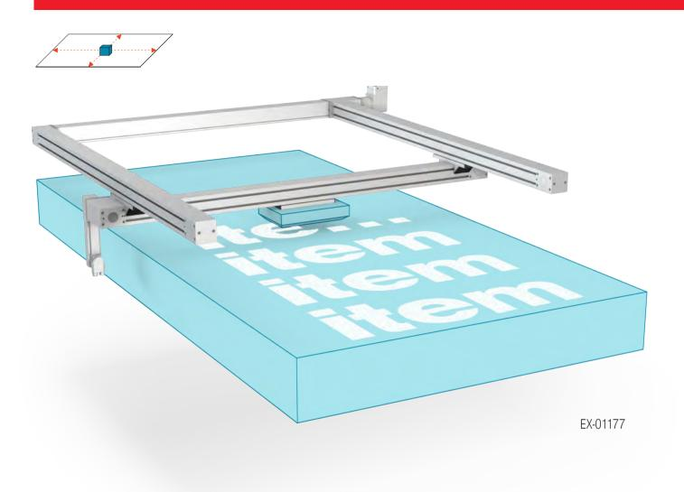
2D flat gantries are perfect for automation tasks in which a tool travels to various points in a single plane. These two-axis solutions are used to print or inspect surfaces, among other things. Tools such as styluses, sensors and print heads need to be moved with precision, often over large distances, which places stringent requirements on the rigidity and synchronous movement of the linear axes in two dimensions.
