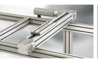
Everything in one housing. The roller elements of the compact item Linear Units KLE run inside the profile. With the exception of the carriage, none of the moving parts can be touched because the timing belt in the guide groove covers the moving elements. This enhances occupational health and safety and reduces soiling on the guides and roller elements.
