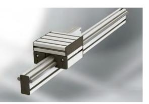
Perfect for vertical movements! Linear Unit LRE 8 D14 80x40 ZS positions itself with a repeat accuracy of just 0.1 mm, even over very long travel distances. As the drive is mounted directly on the slide, it is very easy to build a vertical axis of movement, on which the slide is fixed and the rack is moved vertically. Roller guide D14 ensures that high forces and torques can be accommodated. Linear Unit LRE 8 D14 80x40 ZS can also be used in heavily contaminated environments.
