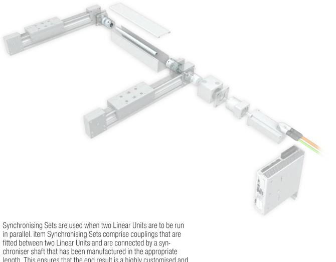
length. This ensures that the end result is a highly customised and flexible design. The Synchroniser Shaft Cover Sets from item are a useful accessory as they stop the synchroniser shaft coming into contact with external influences and keep dirt out, thereby boosting operational reliability.
