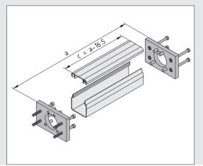
The adapter plates included in the Synchroniser Shaft Cover Set secure the conduit elements between the two timing-belt drives of Linear Units GSF 8 40 R10. Calculating the length:
