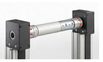
Connecting Shafts are used to provide a torsionally rigid connection between the mechanical drive elements and the corresponding Coupling Half. The Connecting Shafts are inserted into the drive elements until they come up against the stop of the Snap Ring. The clampable Coupling Half is slipped onto the free end of the shaft and clamped axially such that the length of the coupling matches the length of the Coupling Housing, and the Coupling Inserts are not under any axial load.
